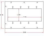
12 Neutrik™ "D" size punchouts for XLR and other type connectors using the same hole pattern.
