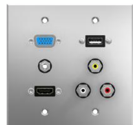
AL2513xx One HD15, 3.5 solder, HDMI, USB A-A and three RCA FT (yellow, red, white)
