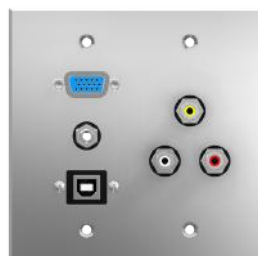
AL2512xx One HD15, 3.5 solder, USB B-A and three RCA FT (yellow, red, white)
