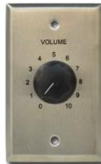
VCSS103xx 1 gang, stainless steel wall plate, xx W, 70V attenuator, silkscreened dial, phenolic knob
